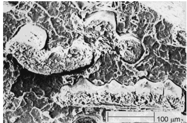
Figure 10 SEM micrograph of RH-PP composites after subjected to being HA at 90°C.
