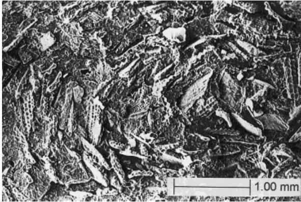
Figure 8 SEM micrograph of RH-PP composites in AR state.
